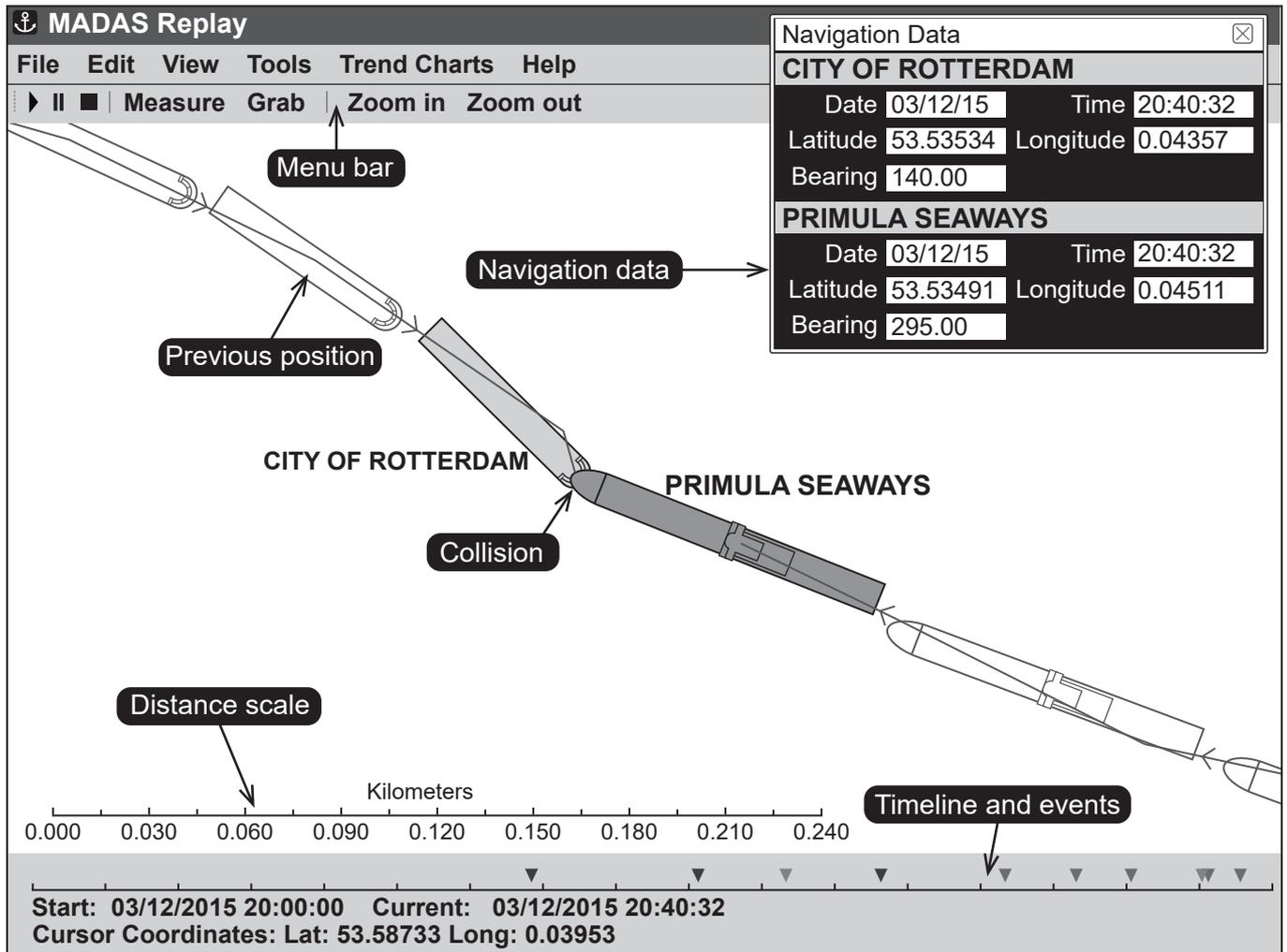
Cruise ships are required to carry a voyage data recorder (VDR), which uses sensors to monitor the conditions in the ship at all times. The data from the sensors is collected and input into a relational database (see **Figure 3**) that is a part of the MADAS system (see **Figure 4**).
